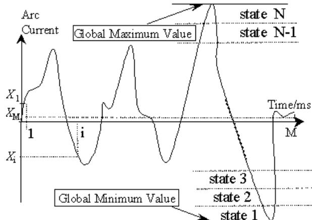
Fig. 1 Illustration of states used in Markov-like model
