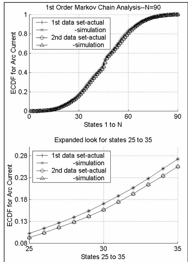
Fig. 3 ECDFs for actual arc current from a first order Markov-like model N=90
