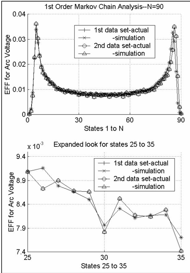
Fig. 4 EFFs for actual arc voltage from a first order Markov-like model N=90
