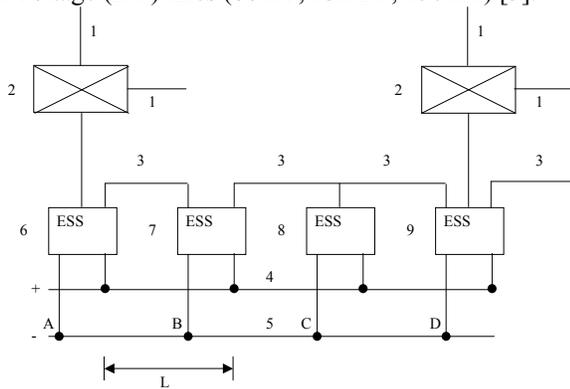
Fig. 1. Diagram of supply of a dc electric traction system. 1) HV ac lines. 2) Electric power substation of ac industrial network. 3) HV ac Primary lines of traction system. 4) Railway dc overhead lines. 5) Rails. 6-7-8-9) Substations of conversion. L) Distance among ESS'.
