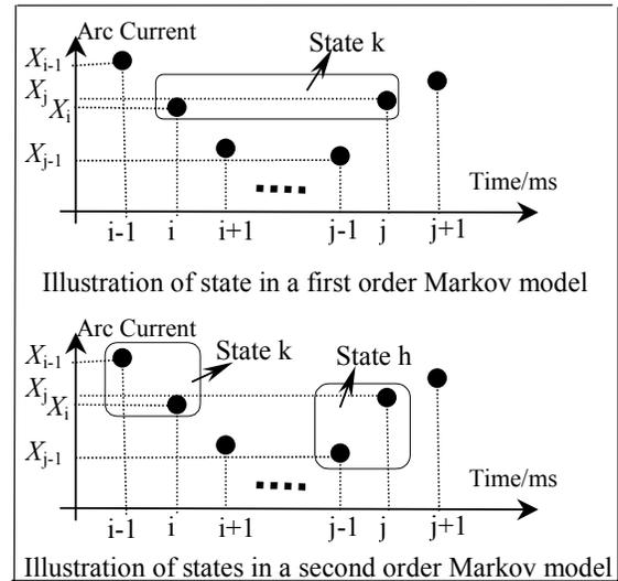
Fig. 5 Comparison of states in first and second order Markov-like model
