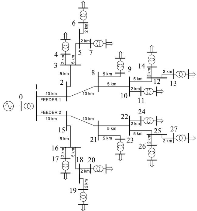
HV equivalent: 110 kV, 1500 MVA, X/R = 10
