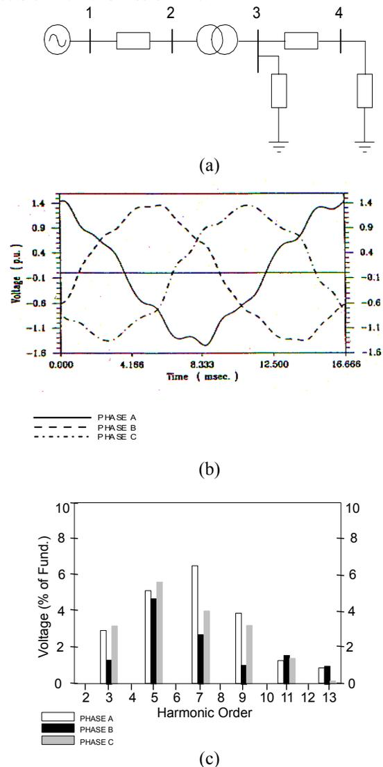
Fig. 2. (a) Test system 1; (b) Voltajes at node 4; (c) Voltaje harmonic content at node 4
