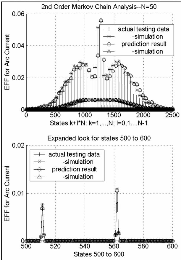
Fig. 8 EFFs for the predicted current from a second order Markov-like model  $N=50$
