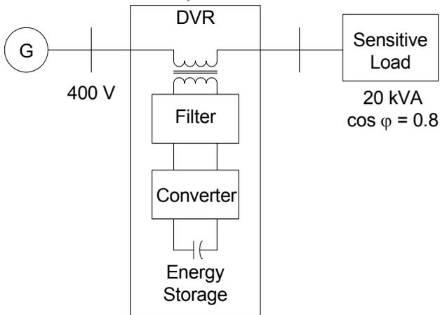
Fig. 6. Mitigation of voltage sags. Scheme of the test case
