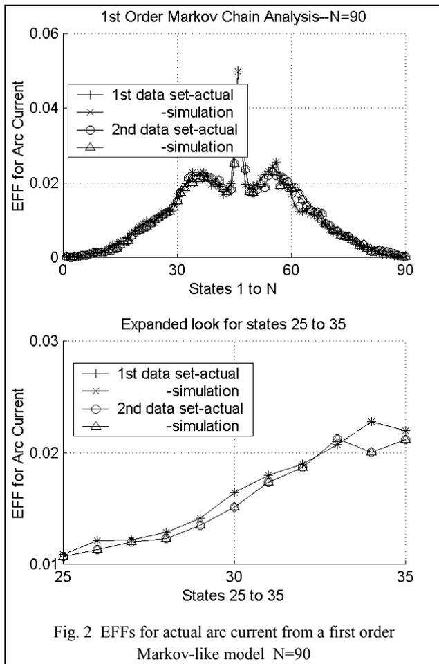
Fig. 2 EFFs for actual arc current from a first order Markov-like model N=90
