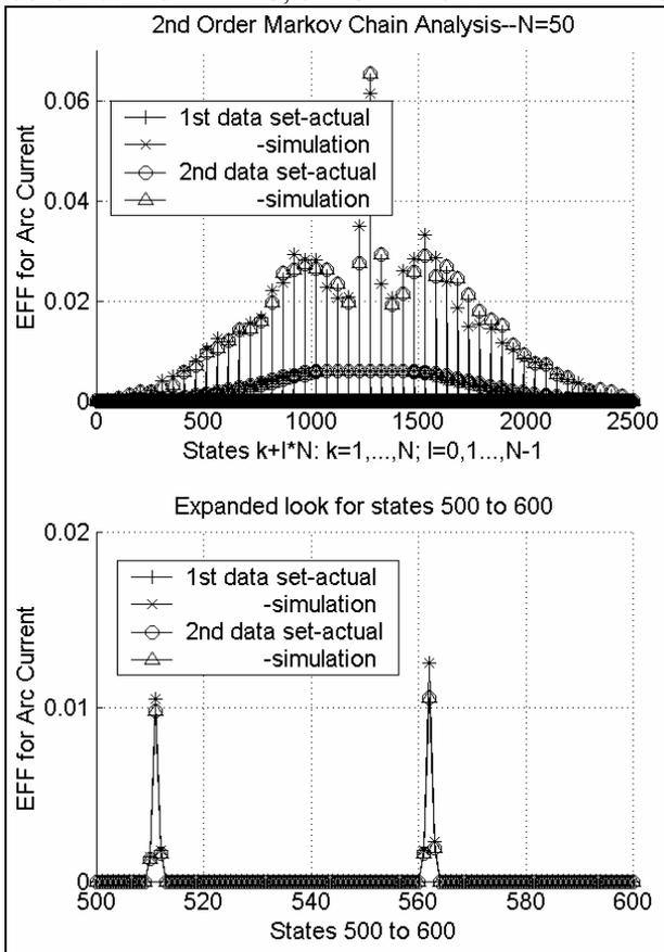
Fig. 6 EFFs for actual arc current from a second order Markov-like model N=50
