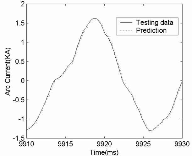
Fig. 7 Waveforms for a part of the predicted and related actual arc current
