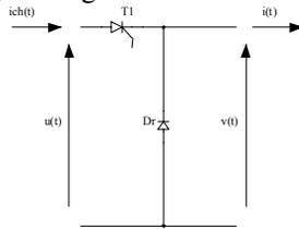
Fig. 3. Simplified diagram of an one-stage converter.
