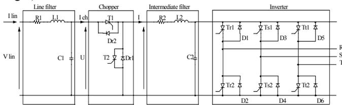
Fig. 4. Circuit diagram of a double-or two-stage converter.
