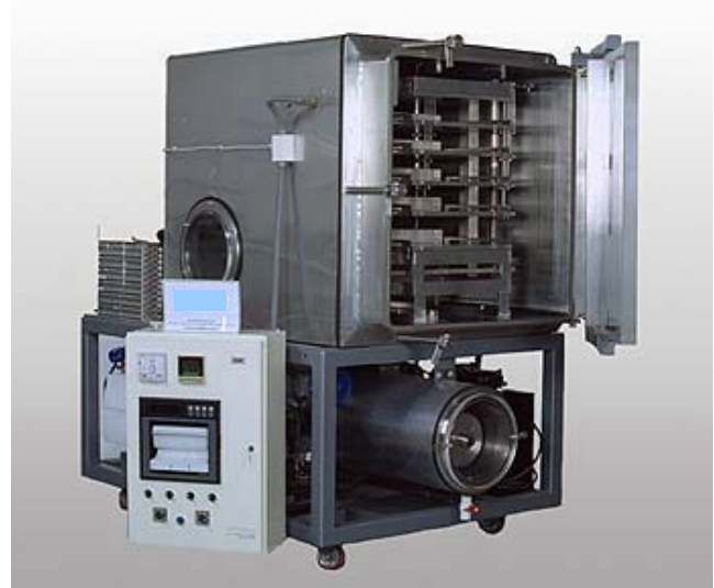
Fig. 10. Typical Pharmaceutical freeze-dryer (Lyophilizer)
